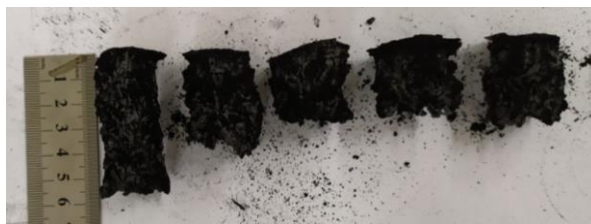
Figure 2. Carbon deposit, consisting of amorphous carbon, SWNTs and MWNTs.
